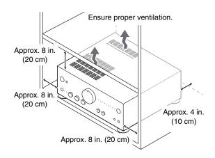
Install the integrated amplifier on a sturdy rack or shelf. Position it so that its weight is evenly dispersed on its four legs. Do not install the integrated amplifier in a place with vibration or an unstable location.
