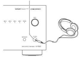
**7** Connect a pair of stereo headphones with a standard plug (1/4 inch or 6.3 mm) to the PHONES jack.
