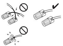
• Don't connect more than one speaker wire to a single speaker terminal. Doing so could damage the integrated amplifier or cause it to malfunction.
