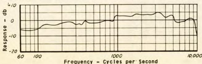
Fig. B. Typical Frequency Response, Series "556" Microphones
